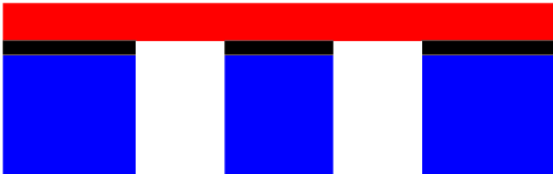
FIGURE 2.4.6B. Example of unallowable “full thickness suspended structure”
