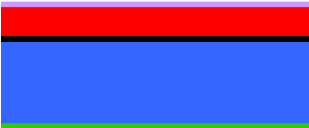
FIGURE 1.2. A phosphosilicate glass layer (PSG) is deposited, and the wafers are annealed at 1050°C for 1 hour in Argon to drive the Phosphorous dopant into the top surface of the Silicon layer. The PSG layer is subsequently removed using wet chemical etching. Note: A Bottom Side Oxide layer is initially present on the starting substrates.
