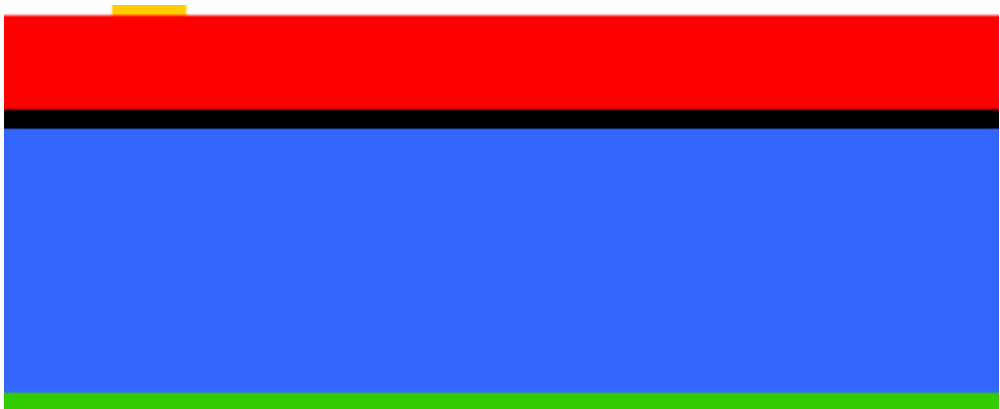
FIGURE 1.3. The wafers are coated with negative photoresist and lithographically patterned by exposing the photoresist with light through the first level mask (PADMETAL), and then developing it. A metal stack consisting of 20 nm chrome and 500 nm gold is deposited over the photoresist pattern by e-beam evaporation. The photoresist is then dissolved to leave behind metal in the opened areas.
