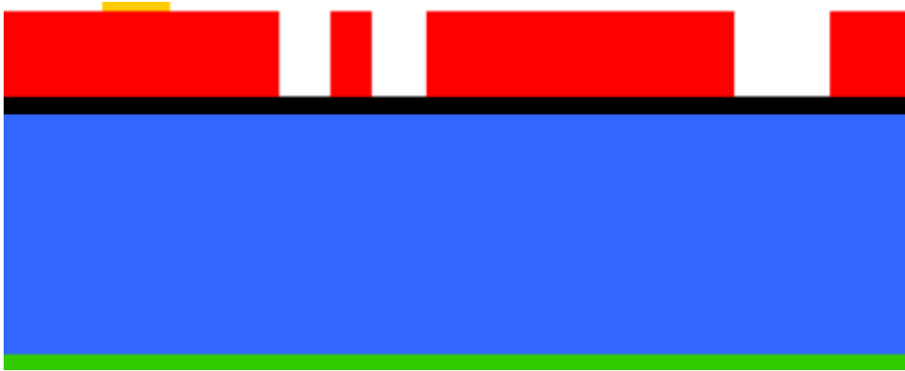
FIGURE 1.4. The wafers are coated with UV-sensitive photoresist and lithographically patterned by exposing the photoresist to UV light through the second level mask (SOI), and then developing it. The photoresist in exposed areas is removed, leaving behind a patterned photoresist mask for etching. Deep reactive ion etching (DRIE) is used to etch the Silicon down to the Oxide layer. After etching, the photoresist is chemically stripped.
